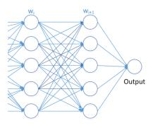
Figure 4: Fully Connected Layer
